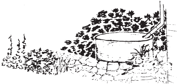
Downspout into dry well
